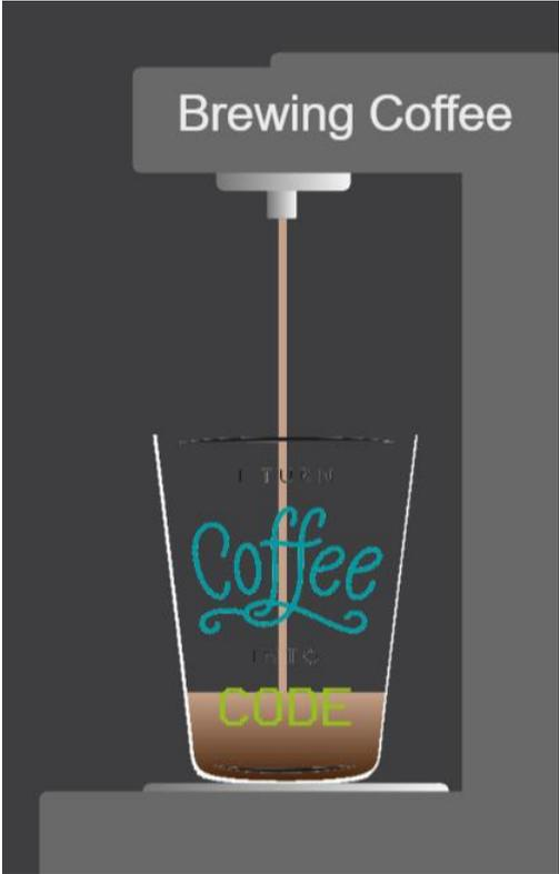
If the second button is pushed, the brewing coffee mode is activated. On the web visualization a cup of coffee will be filled. The level of the coffee cup is also shown on the LEDs of the AXL SE DO16/1 module.
